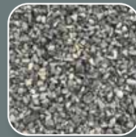
3/4" CLEAN CHIP GRAVEL
